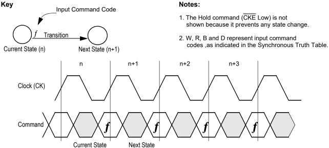
Current State and Next State Definition for Pipeline and Flow Through Read/Write Control State Diagram
