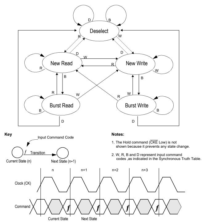
Current State and Next State Definition for Pipeline and Flow Through Read/Write Control State Diagram
