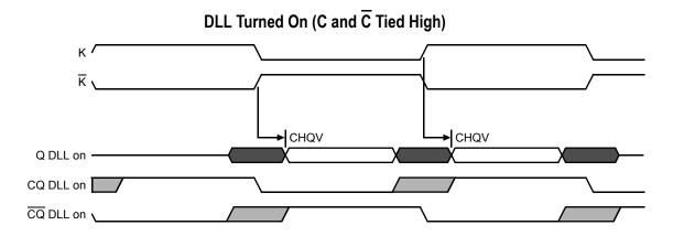
The following figure shows a simplified timing diagram for the SigmaQuad-II and includes the use of C and  $\overline{C}$ .
