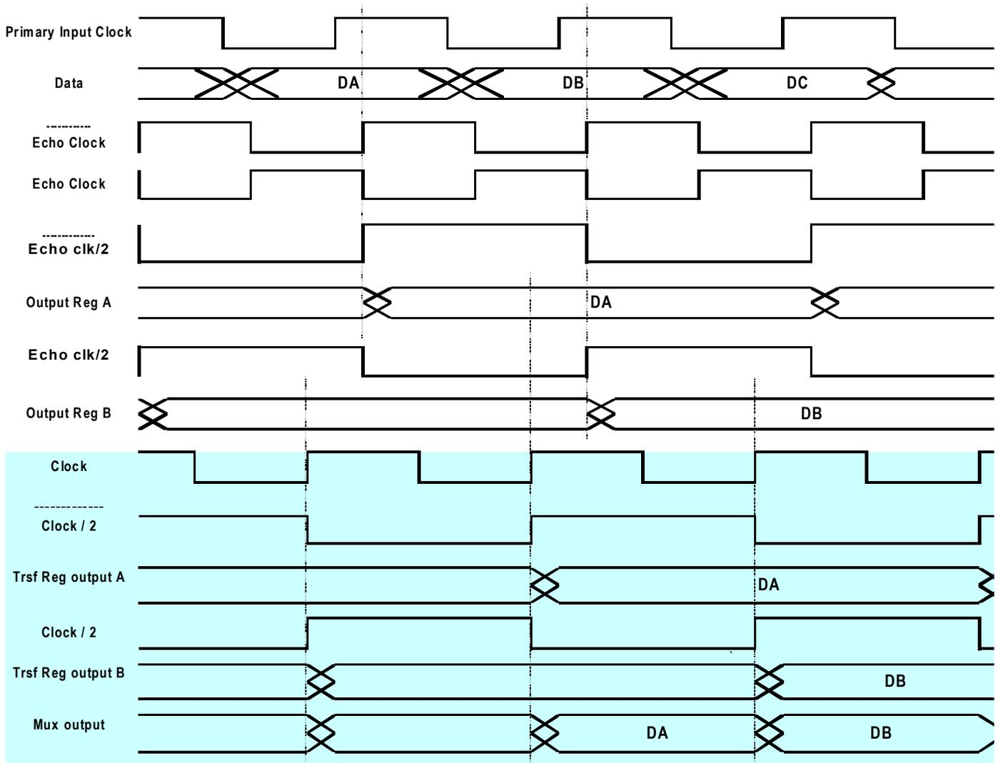
**Figure 5: SDR Timing**
